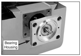
Figure 67. Y-axis bearing housing.
